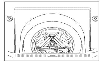
3. Turn the nut holding the jack package container counterclockwise and remove it. Then remove the jack and wheel wrench.
